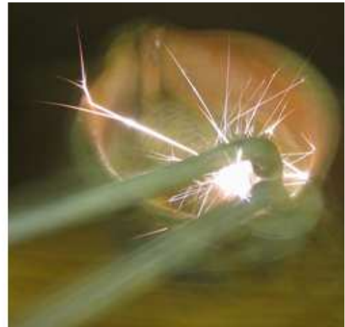
78: Cutting Torch Sparkers: These little spring-loaded sparkers (which have replaceable flints) are used for lighting gas torches, but they will also light most tinders as well as any other spark-based technique.
