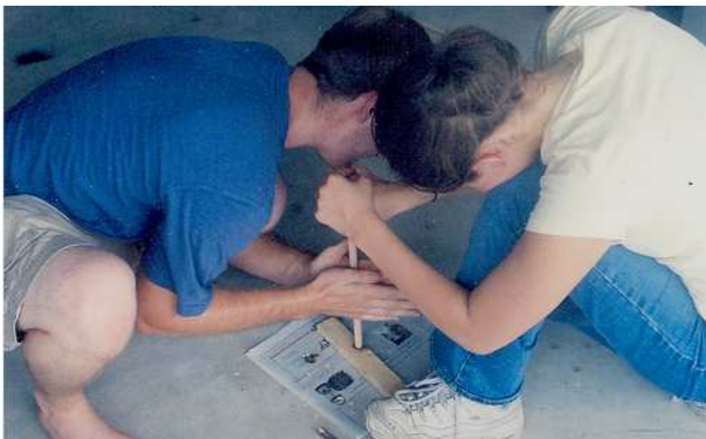
32: Team Hand Drill: Two people can work together to keep a hand drill spinning, to reduce fatigue.
