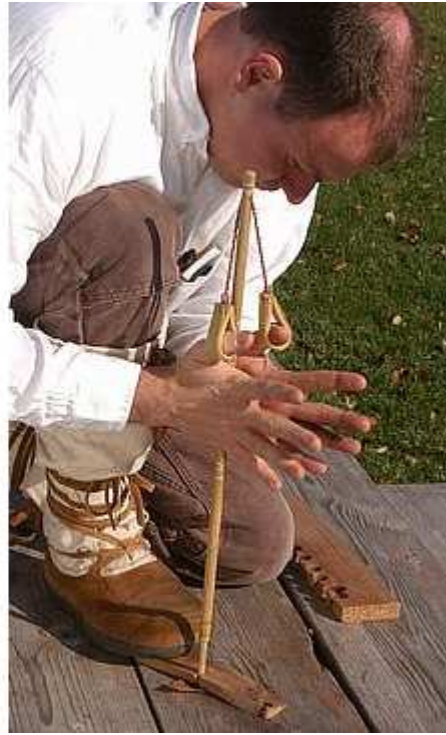
33: Thong Hand Drill: Tying a cord (with thumb loops) to the top of the spindle of a hand drill allows you to increase downward pressure as you spin the spindle, and your hands don't travel down as you spin, making this a much easier technique to use.
