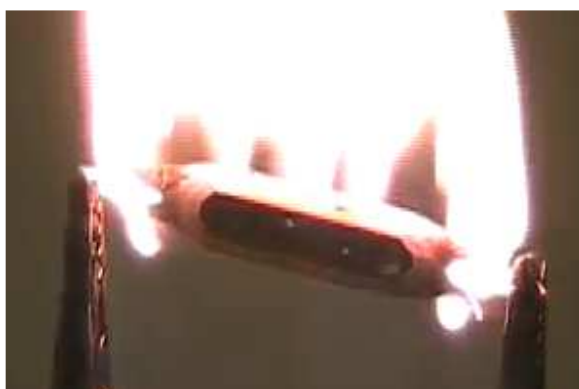
83: Electricity and Battery Power (electricity and a wooden pencil): If you run enough electricity (such as household 120 volt AC) through a short section of wooden pencil, the pencil lead will act as a resistor and generate enough heat to ignite the wood.
