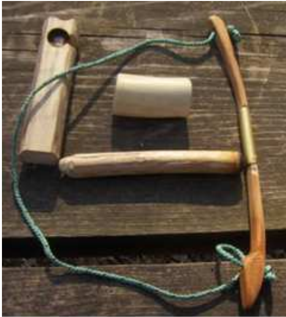
44: Fire Bow Drill (collapsible): Since the bow of a bow drill doesn't flex like an archery bow (it just holds both ends of the cord), you can make a collapsible bow that can be stored in a small space. Like a collapsible spindle stick for a hand drill, the collapsible bow can have a socket made from bamboo, or metal tubing.
