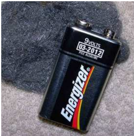
80: Electricity and Battery Power (using steel wool): Steel wool is easy to set on fire with electricity. If a bit of steel wool is spread apart (to increase surface area), even a weak battery will cause it to spark and burn, and it can be blown into a flame with little effort.
