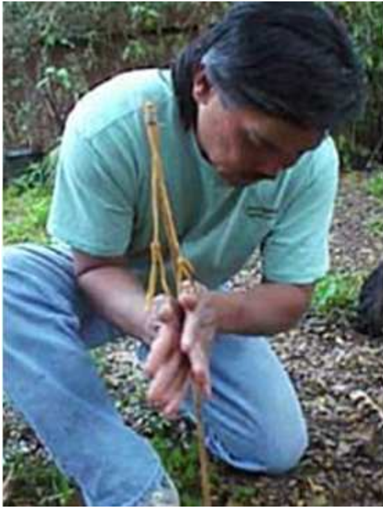
33: Thong Hand Drill: Tying a cord (with thumb loops) to the top of the spindle of a hand drill allows you to increase downward pressure as you spin the spindle, and your hands don't travel down as you spin, making this a much easier technique to use.
