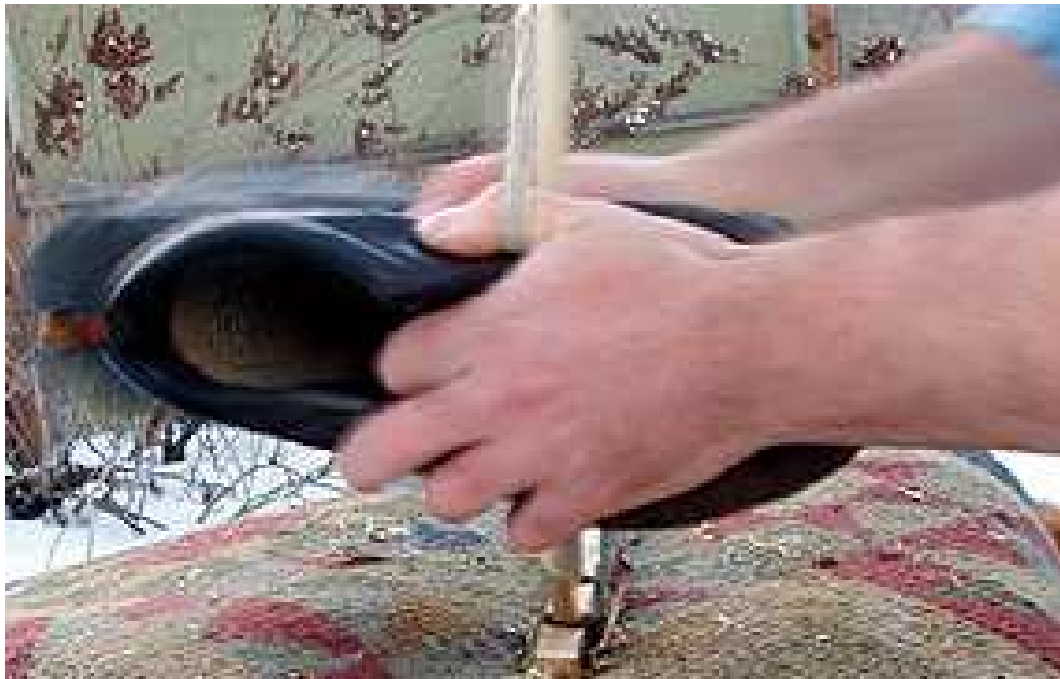
34: Shoe Hand Drill: Spinning the hand drill can cause your palms to ache. One way to avoid this is to hold a pair of shoes against the spindle, so that the soles absorb all the punishment. Use a cord with thumb loops as well (try the shoelaces). Other objects could also be used, if you don't have shoes, such as short lengths of 2x4 lumber (roughen the contact surfaces), or pads cut from an automobile tire.
