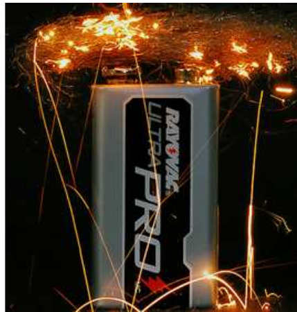
80: Electricity and Battery Power (using steel wool): Steel wool is easy to set on fire with electricity. If a bit of steel wool is spread apart (to increase surface area), even a weak battery will cause it to spark and burn, and it can be blown into a flame with little effort.
